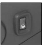
You can lock or unlock all doors of your vehicle from the driver's or front passenger's door lock switch.
